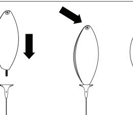
**1.** Line up the *balloon cup* (B) with the grooves on the side of the corresponding *stem* (C). Snap cup into place. Repeat for all the stems. **2.** Attach the *balloon* (A) onto the *stem* (C) by lining the silver push pin located on the black piece at the bottom of the balloon with the hole on the bottom of the appropriate cup. Lock the balloon in place. Repeat for all balloons.
